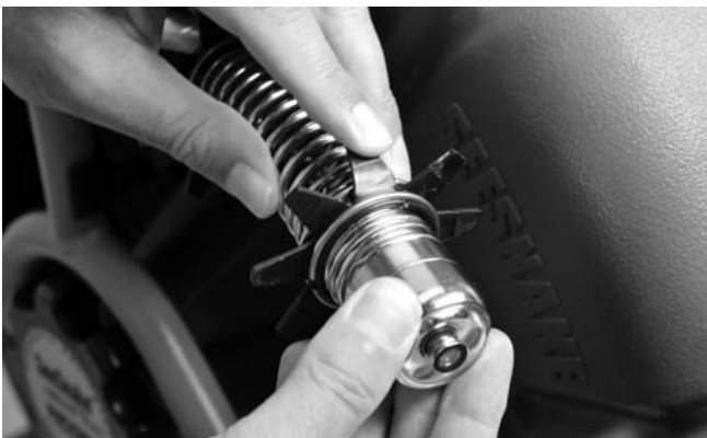
Figure 14 – Pre-stressing The Flanges
