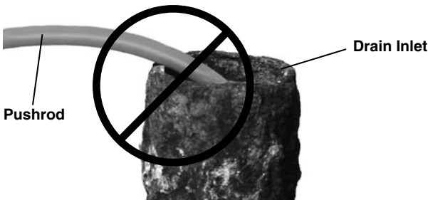
Figure 33 – Avoid Pulling At Sharp Angles
