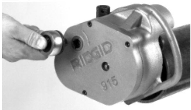
Figure 7 – Ratchet in Input Drive
