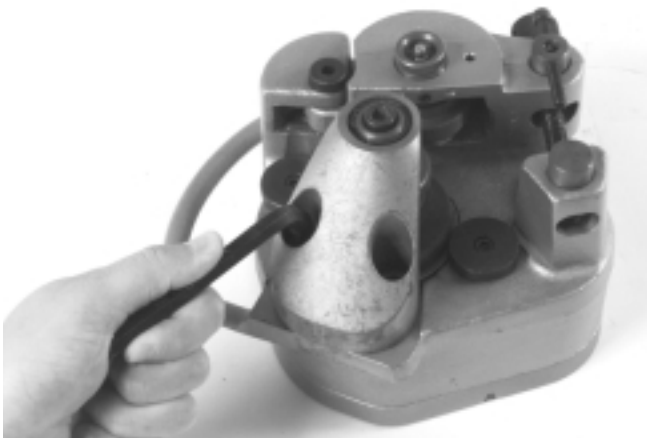
Figure 12 – Installing Drive Rolls
