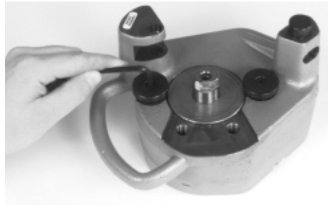
Figure 17 – Installing Copper Stabilizer Pad
