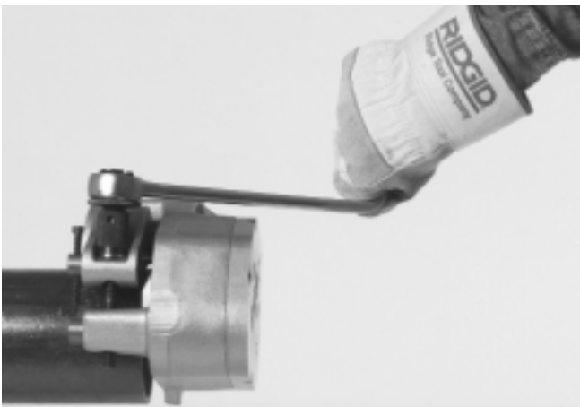
Figure 5 – Ratchet in Feedscrew
